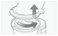
· When moving the appliance, do not lift by grabbing the feeding tube. Always lift the appliance by grabbing the body or handle.
