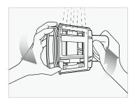
Thoroughly rinse the inside and outside of the screen under running water.
