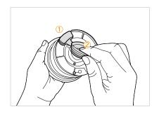
The silicone cover is removable for cleaning. After cleaning, place the silicone cover in regular sequence on as shown in the picture.
