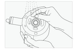
Under running water, clean the auger with a sponge. Use the tip of the cleaning brush to dislodge any residue from the crevices of the auger.
