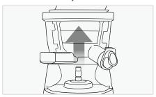
Remove the auger, screen, and wiping blades from the juicing bowl. Clean with provided brush. Immediately clean the juicer after each use. If juice is allowed to dry, it will cause a build-up of organic residue. This is both unsanitary and can affect the juicer performance.
