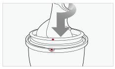
Note | The auger needs to be locked in place in order for the drum lid to close properly.
