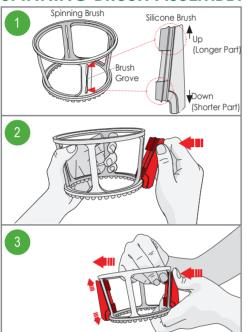
Check the groove of the spinning brush and the direction of silicone brush.
