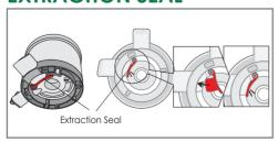
The silicone pulp stopper is located at the bottom of the Juice Bowl. Before use, make sure the seal is closed. For cleaning, open the extraction seal and wash out trapped food.
