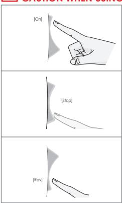
To STOP the operation, press the [Rev] button quickly. The auger will rotate slowly then stop. After the auger rotation stops completely, you can press [ON] to continue operation as normal or hold down the [Rev] button to push ingredients upward.
