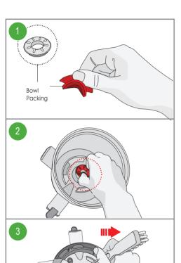
As shown to the left in the dotted circle, let the protrusion part on the bowl packing face upward and hold it, like pinching, with your thumb and index finger.
