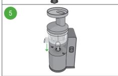
Mount the assembled juice bowl chamber onto the motor base.
